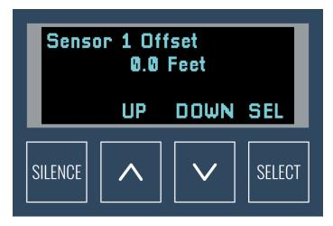
Add an offset to the analog sensor reading.
