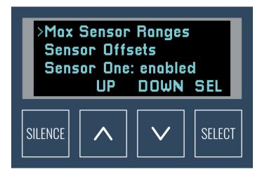
The Settings Menu is where you can configure the alarm. It is passcode-protected if enabled.
