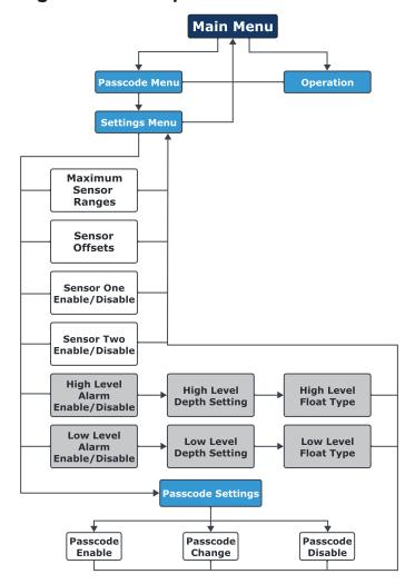
From the Settings Menu, the following parameters may be changed: Maximum Sensor Ranges, Sensor Offsets, Sensor One Enable/Disable, Sensor Two Enable/Disable, High Level Alarm Settings, Low Level Alarm Settings, Passcode Settings.
