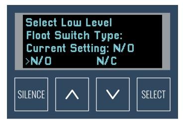
Change the float switch type between Normally Open and Normally Closed for the Low Level float switch.
