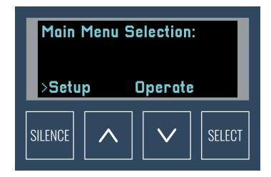
Navigate between the Settings Menu (Setup) or the Operation Menu (Operate).
