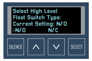
Change the float switch type between Normally Open and Normally Closed for the High Level float switch.
